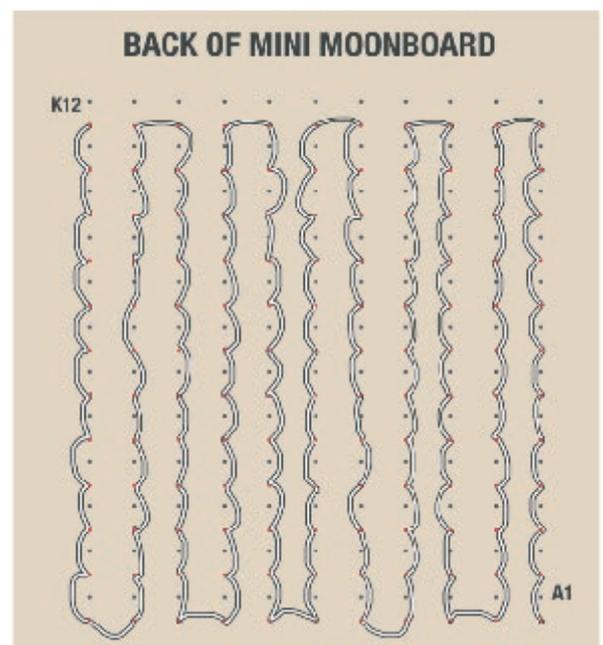
Once you have used all of the LED's in string A, connect the LEDs from string B to set A using the push fit connector, and continue installing in the zig-zag pattern.
