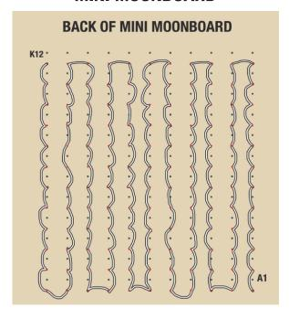
Once you have used all of the LED's in string A, connect the LEDs from string B to set A using the push fit connector, and continue installing in the zig-zag pattern.
